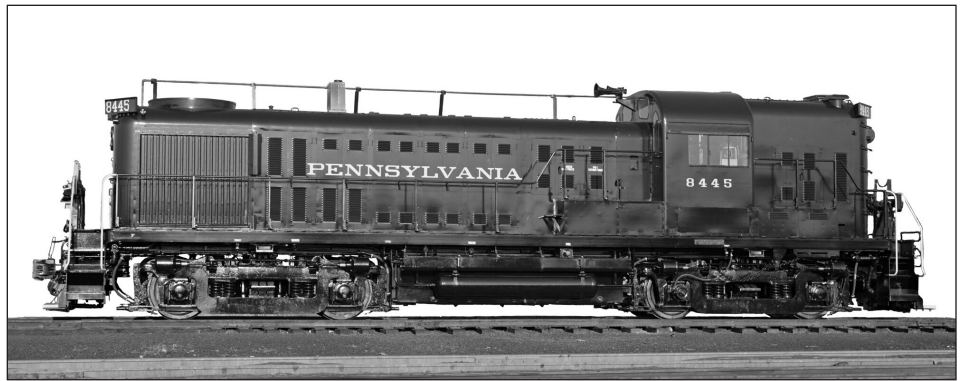
Builder's photo of Pennsylvania Railroad Alco RS-2 8445, one of five similar units built with a high short hood to accommodate both dynamic brakes and a steam generator for passenger service. Built in 1953, it was renumbered 5569 after the 1968 Penn Central merger. It was traded to Lehigh Valley in 1970 where it became 211. It was rebuilt by Conrail in 1979 and became 9900. Retired in 1981, it was acquired by several museum members and donated in 1986. It was restored to LV colors in 1990 and remains an important part of our museum's operating fleet. —ALCO HISTORIC PHOTOS
