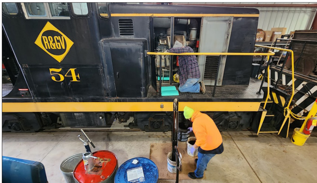
ABOVE: On January 10, Greg Lund and Justin Carmona perform an oil change on R&GV 54, a General Electric 60-ton switcher built in 1959 for the U.S. Army.
