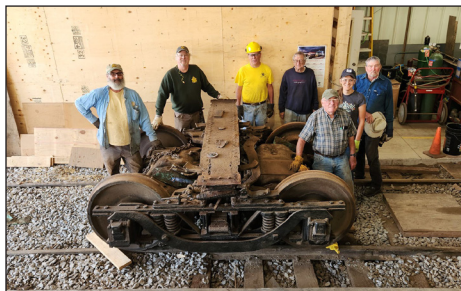
LEFT: Rochester Subway Car 60's rear truck was carefully removed from the body so the bolster can be repaired on September 19.
