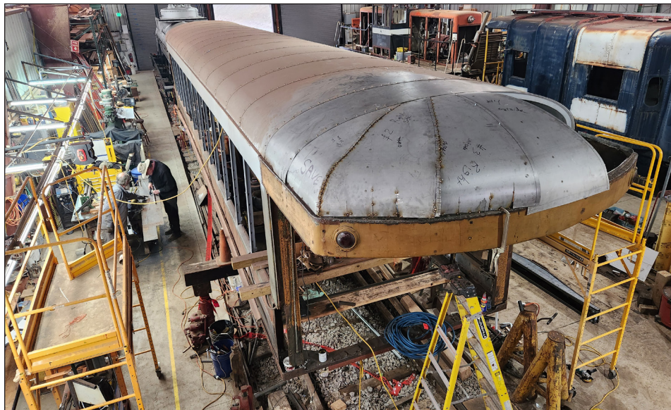
ABOVE: Sheet Metal Workers Union Local 46 apprentices are making good progress on fabricating the new curved roof at the south end of Rochester Subway Car 60. At the same time, Bill Marcotte has been leading the fabrication of a new rear truck bolster.
