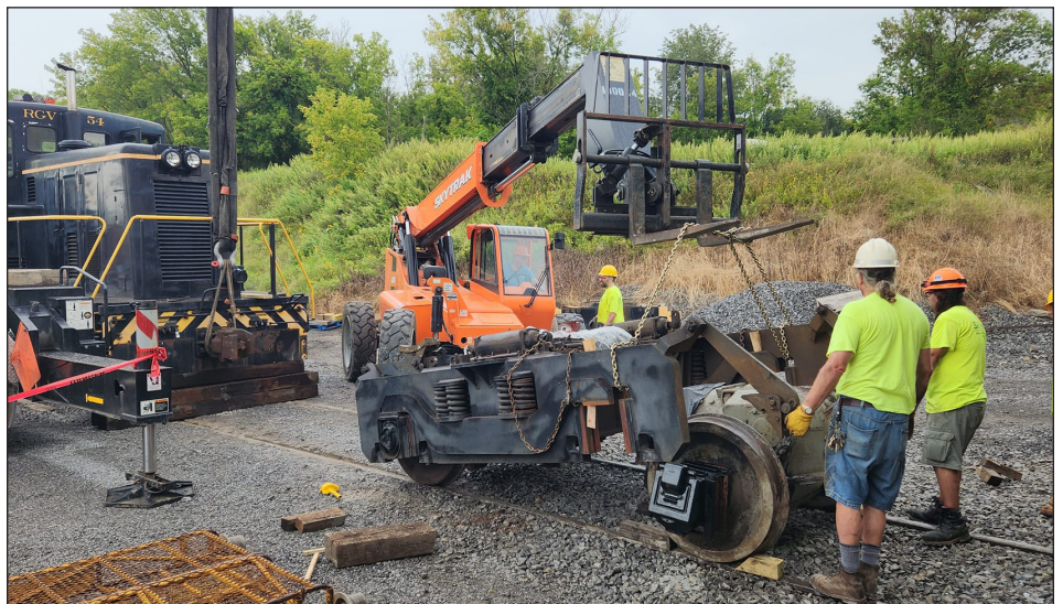
TOP: "The Big Lift" took place on September 7 to swap three of the four axles on R&GV 54 with replacement traction motor combos. The C.P. Ward crane lifts one end of the locomotive so the truck can be rolled out. ABOVE: We rented a heavy-duty forklift to perform the lift on the truck frames so the new traction motor combo units could be installed. See page 4 for details.
