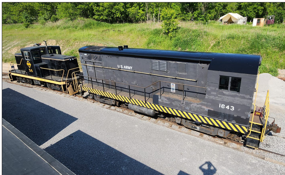
Volunteer Chuck Whalen has completed putting a new coat of paint on the roof of our Fairbanks Morse H12-44 1843. Sam Rosenberg has been working on updating the electrical systems inside to make operation more reliable in the future.
