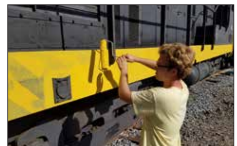
BELOW: Kurtis Hooey and his friend Daniel Gardiner have been touching up some of the rust spots on USA 1843, including repainting the hazard strips on the sill. The Fairbanks-Morse H12-44 diesel was built in 1953, and came to our museum in 1993.
