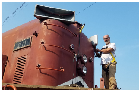
ABOVE: Bill Marcotte fabricated new “bug eye” number boards for the high hood of LV 211. The originals were removed by Conrail in 1979.
