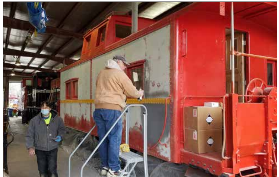
BELOW: Charles Bell has been applying a skim coat of body filler and sanding it smooth to prepare Lehigh Valley 95100 for its finish coat later this summer.
