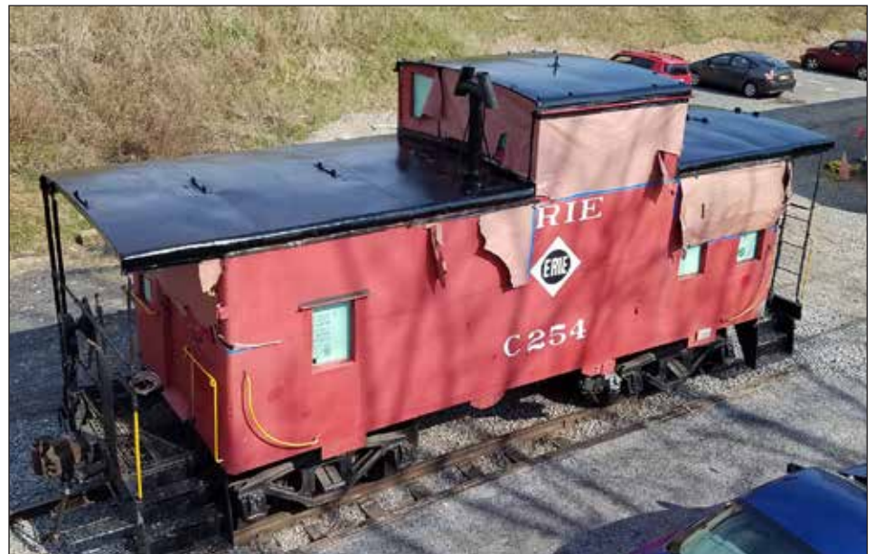
ABOVE: Justin Carmona, Jackson Glozer, and Charles Rothbart apply masking on April 17 to protect the body while the roof is sandblasted.
