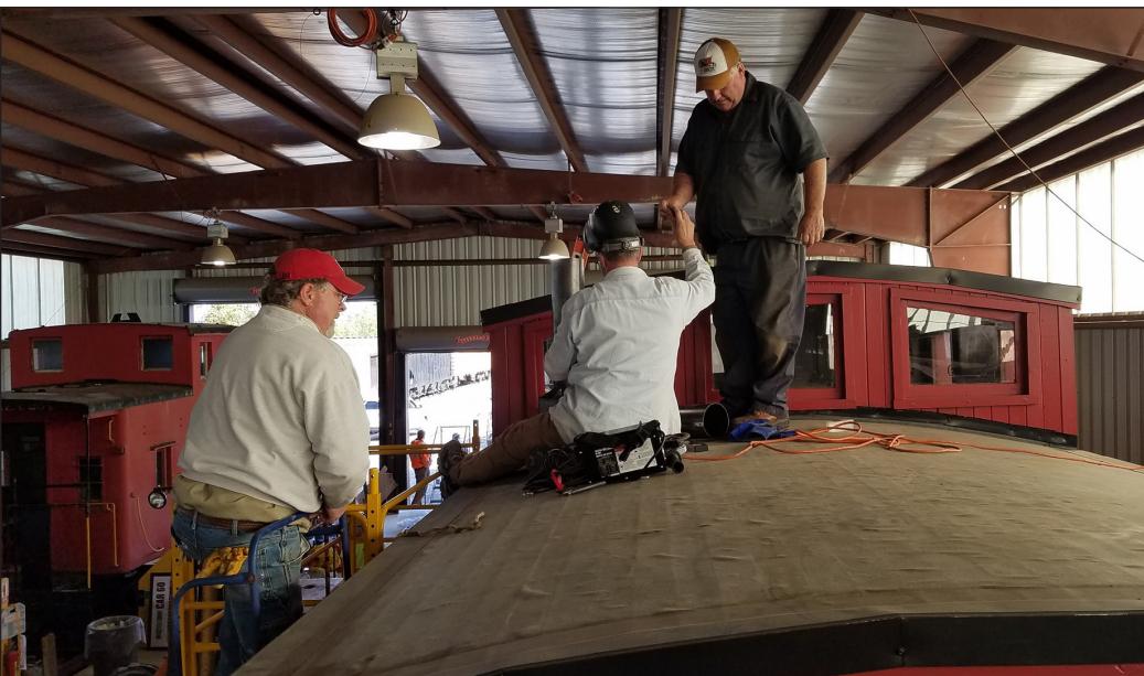
LEFT: Jeremy Tuke, Bill Marcotte, and Charlie Marks up on the roof of Buffalo, Rochester & Pittsburgh 280, carefully cutting holes in the roof for the new chimney fabricated by Bill, and for a cupola signal lamp.
