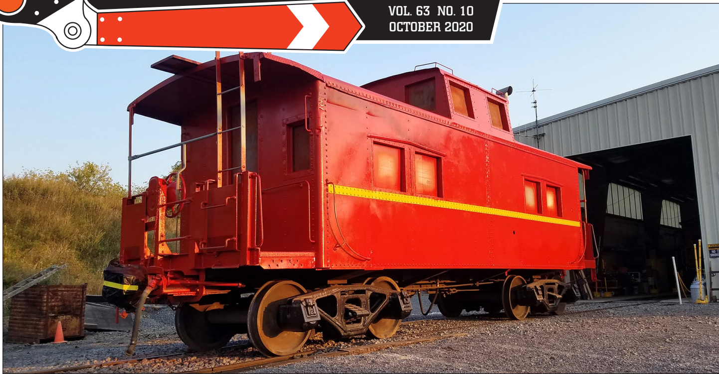
The first coat of red paint has been applied and the masking has been peeled back to reveal the yellow stripe on October 9. PHOTO BY OTTO M. VONDRAK
