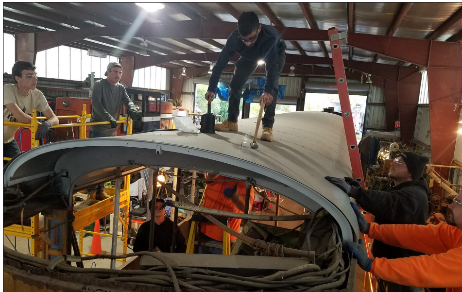
ABOVE: Thanks to Sheet Metal Workers Union Local 46 and their apprentice program, work is wrapping up on the main portion of the roof of Rochester Subway Car 60.
