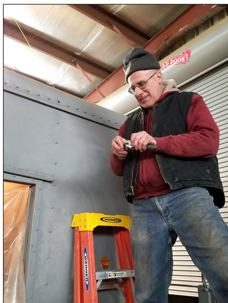
LEFT: Rob Burz prepares to thread a blind rivet to complete a roof repair on LV 95100.
