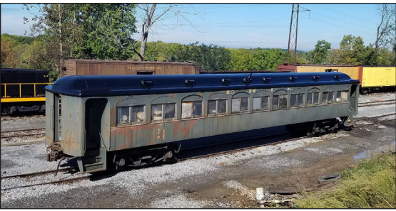
ABOVE: Thanks to a generous donation by the Stillwell Family, we hired a local contractor to powerwash, sandblast, prime, and paint the roof of our Erie Stillwell Coach no. 2328.
