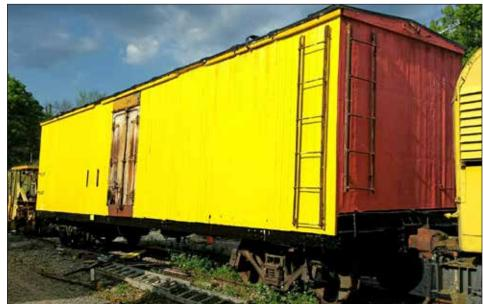
Significant work took place throughout the month of June to remove rotten siding from the west side our Fruit Growers Express refrigerator car. Work was in progress on June 24 (TOP) and was nearing completion on July 13 (ABOVE). The car will get a fresh coat of paint and then placed on display on Track 6 in the upper yard. Thanks to David Petersen and his volunteers for completing this important work to stabilize this wood-bodied freight car.
