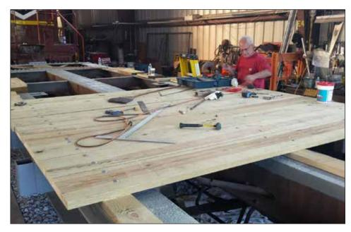
Rob Burz is heading up the project to transform our former Army 40-foot flatcar into an open-air passenger carrier. Several volunteers helped prep and prime the steel frame before the first wood decking was applied in mid-July. Once the deck is complete, the benches, sides, and roof will be installed. Thanks to David MonteVerde for his significant donation towards the deck lumber.
