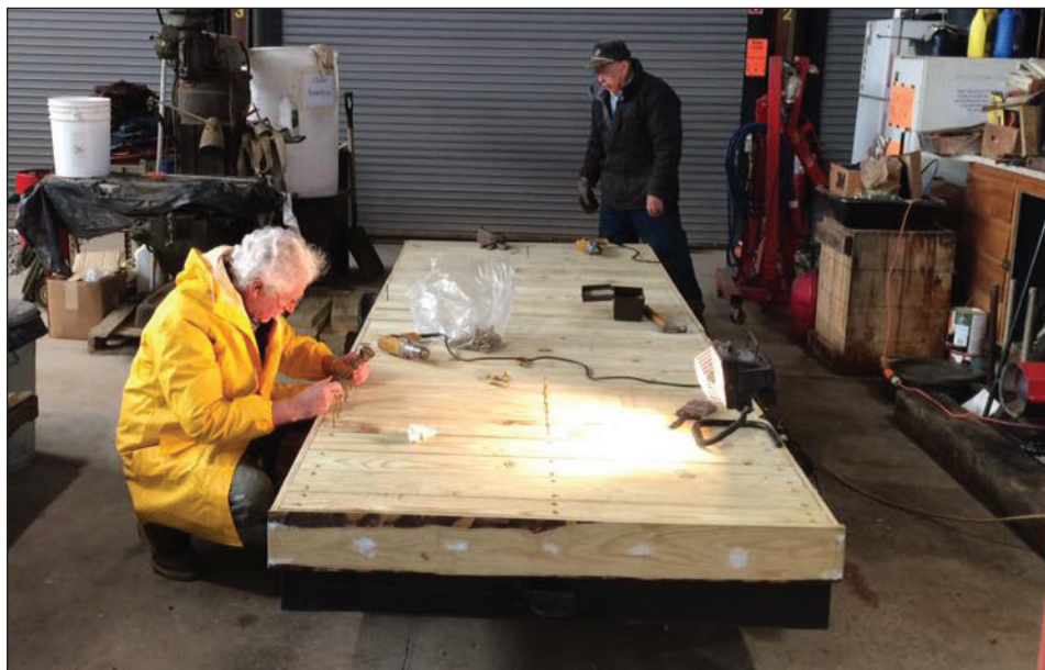
Volunteers Joel Shaw and Norm Schaddick continued working on the wood deck of our new homebuilt TC trailer. The next step will be to add plywood sheathing to help protect and strengthen the deck. This new trailer will be used to transport materials in support of our track gang.
