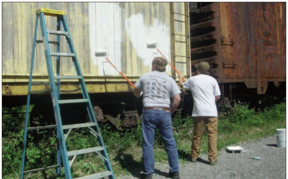
ABOVE: Mark Skipworth and Adam Lloyd pitched in to scrape, prime, and paint our FGE and MDT reefers on May 23, 2015. The other sides will be painted later in the season. LEFT: Lynn Heintz and Rand Warner were scraping the Pennsylvania Railroad hopper on June 6 to prepare it for primer. BELOW: Joe Nugent is putting fresh paint on RG&E 1950. These are not the final paint jobs, but it will help preserve what we have until we have the resources to attempt a full-on restoration. OTTO VONDRAK PHOTOS
