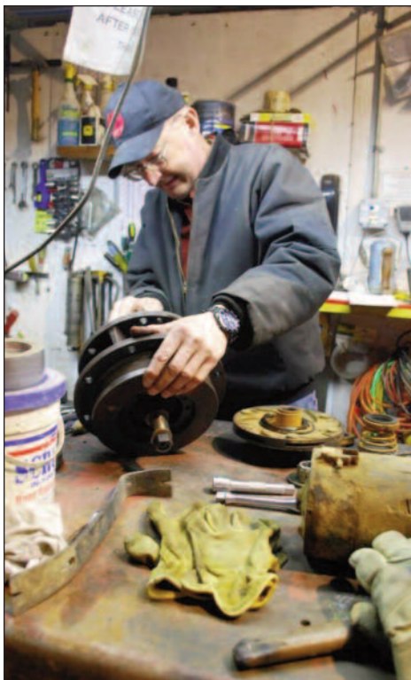
Volunteer Dave Boswell tears down the old water pump from Lehigh Valley 211 to make some repairs that will help bring her back to active service. May 6, 2014. JOE NUGENT PHOTO
