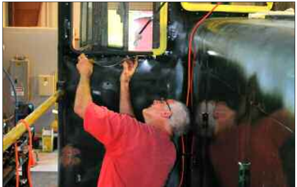
Volunteer Chris Hauf has been spearheading our efforts to complete the final finish painting on RG&E 1941 over the last few weeks. (TOP) It's not as simple as opening the can and applying a coat of paint, the proper amount of hardeners and thinners must be mixed together when working with professional finishes. Volunteer Rob Burz (ABOVE) helps carefully mask off parts of the locomotive that are not to be coated with Brewster Green. PHOTOS BY JOE NUGENT
