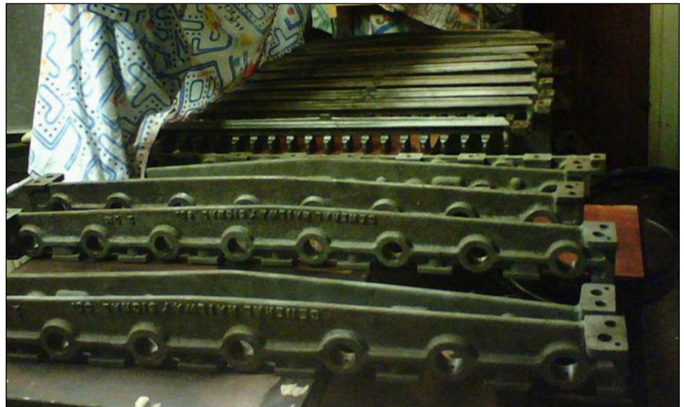
Volunteer Mike Dow has been taking the salvaged parts from the old Niobe tower and slowly restoring and reassembling them into a working machine. On Mike's workbench we find some restored lever latch handles and numbers (TOP). Here we see some parts of the locking bed cleaned and organized (ABOVE). PHOTOS BY MIKE DOW
