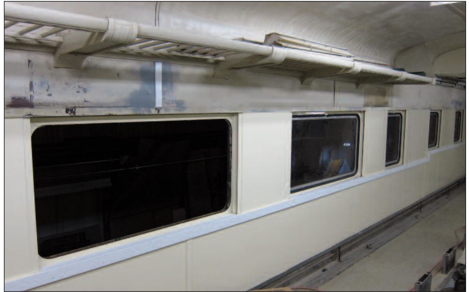
Former New York Central coach 2567 is sporting new paint, including the window openings and four permanently installed windows! PHOTO BY CHRIS HAUF
