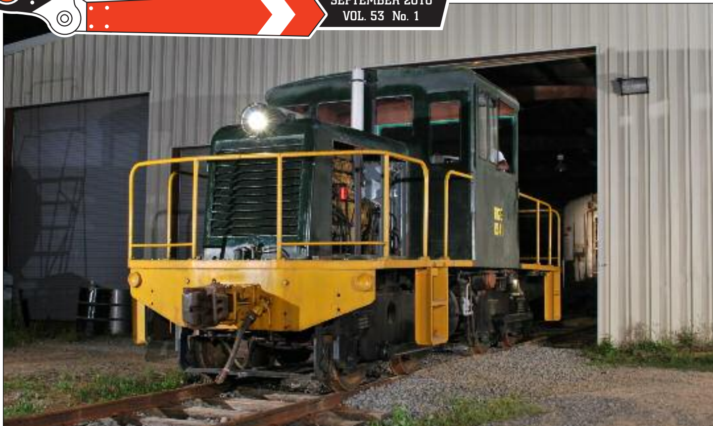
(ALMOST) READY FOR MY CLOSE-UP: RG&E 1941 poses outside the restoration building on a dark August night. This photo was taken during the night time photo shoot after the August chapter meeting. Recent progress includes the installation of radiator louvers, headlights, and a polished bronze bell. It is hoped that reassembly can be completed this winter, and this project will finally leave the shop! PHOTO BY JOE NUGENT
