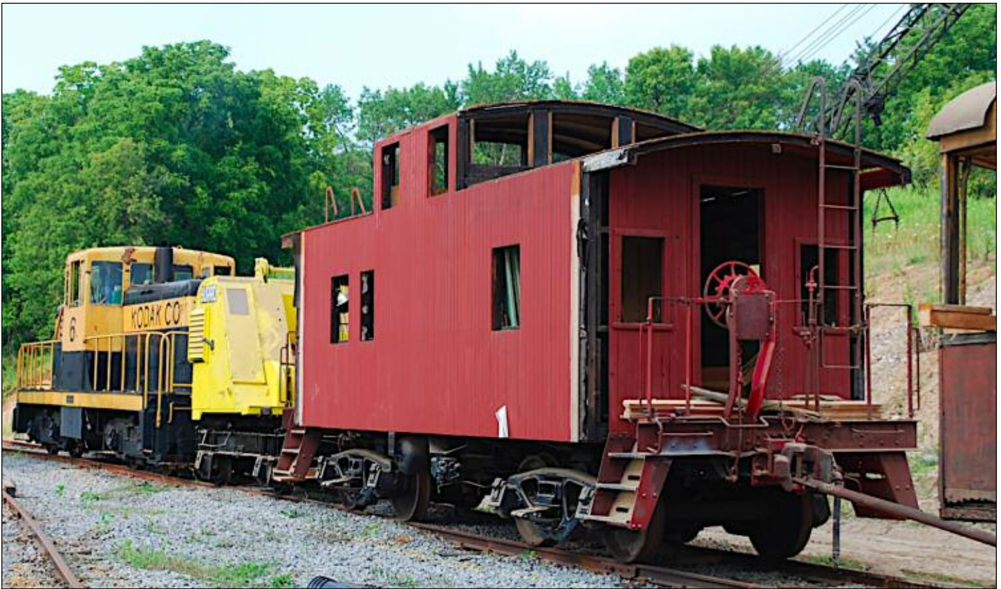
Some of our historic equipment was rearranged and switched out of our Restoration Building on August 15, 2009. Currently in the middle of a multi-year restoration and rebuilding to its 1930s appearance, B&O C-2631 will one day emerge as Buffalo, Rochester & Pittsburgh 280. Project manager Chris Hauf has been coordinating the majority of the work, which involves not only replacing the outside sheathing, but recreating the original interior fixtures and furnitures. As part of B&O's I-10 class, this series of wooden caboose served until 1977. PHOTO BY JOE NUGENT
