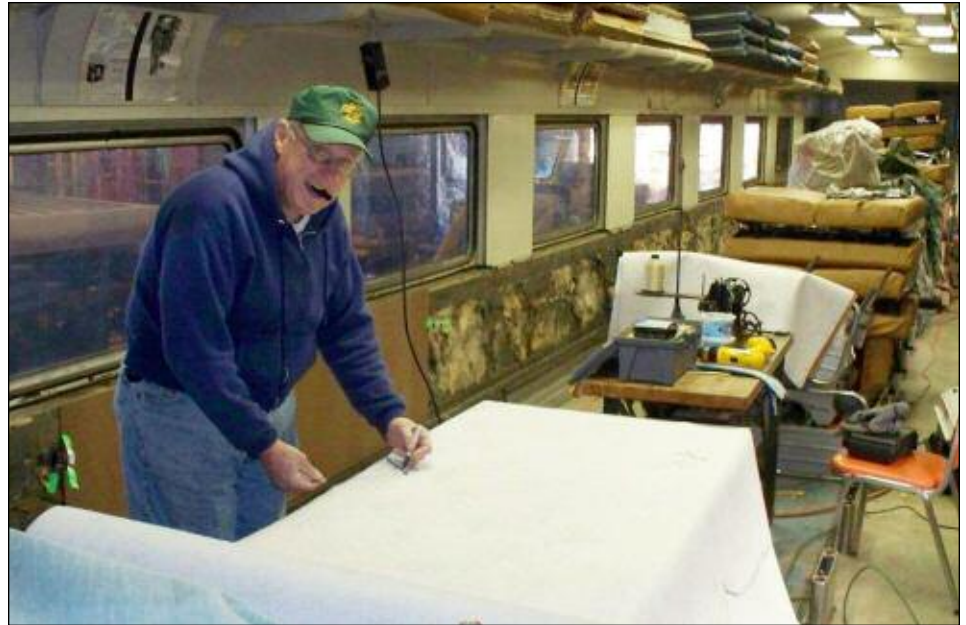
DON'S UPHOLSTERY SHOP: Don Wawrzyniak works on new seat-back upholstery for one of the Chapter's ESE cars on January 16, 2010. Note piles of completed seat backs and bottoms already sporting new covering. PHOTO BY JEREMY TUKE
