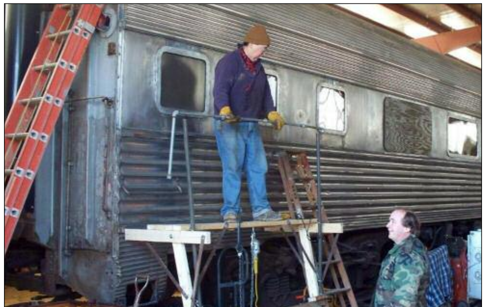
SAFETY FIRST: Dale Hartnett makes progress on new work platform designed to make window replacement efforts safer and easier. Volunteer Jim Bridger assists Dale with the construction on January 16, 2010. PHOTO BY JEREMY TUKE
