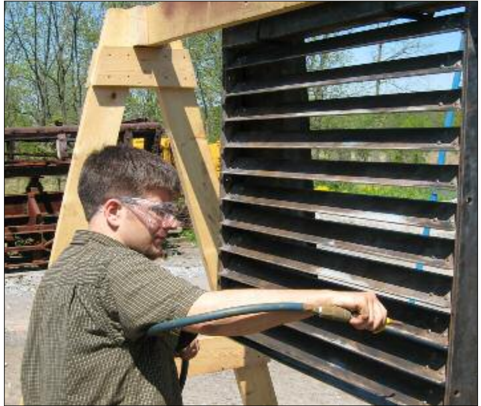
To complete the cosmetic restoration of Rochester Gas & Electric GE 45-tonner #1941, the priming and finish painting of the radiator louvers has to be done before they can be reinstalled. Once in place, then the engine can be painted. Project manager Joe Nugent (above) cleaned the louvers up after insuring the mechanisms were freed up. He moved the assembly down to the Industry depot parking lot where Chris Hauf took over to prime and paint them. PHOTO BY CHRIS HAUF
