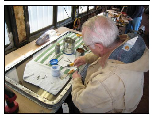
**Volunteer, Bill Blaesi,** is working on the glazing replacement for the museum's 'Empire State Express' coaches. Here Bill is re-tapping the holes that hold the window module together after installing new glazing. This is one of the final steps in rebuilding a window module. [Caption and photo by Chris Hauf]
