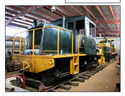
Tonners in the building! With Track #8 further extended in the Restoration Building, both GE 45-tonner RG&E #1941 and GE 80-tonner Eastman Kodak Company #6 rest INSIDE the building for work this winter. [Chris Hauf photo & caption]
