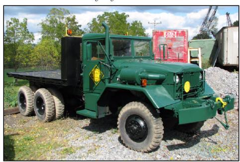
Over the past few weeks. Dan Waterstraat has worked to convert one of our Army 6x6 trucks over to a flat bed using the flat bed deck from one of our out of service trucks. Here the truck is seen with its new flat bed, all new paint, and new R&GVRRM logos cut and applied by Chris Hauf using the Chapter's sign vinyl cutting system. This truck will add real capability to the museum for MANY projects. Nice work Dan!
