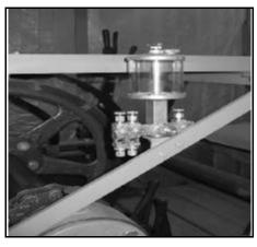
Above With a gas-mechanical chain drive locomotive, keeping your chains properly oiled is a must. To insure our Plymouth BL's chains stay lubricated, Kevin Klees has fabricated this chain oiler setup which will feed brushes mounted on the various drive chains. [Chris Hauf photo and caption]
