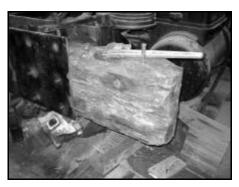
Here we see the large wood beams of Vulcan #12's pilot beam exposed. There are two beams that make up the pilot, and are badly rotted. The beams are approximately 9.5" square and stacked one on the top of the other. Plans are to replace these large wood beams with three railroad switch timbers. [Chris Hauf photo and caption]
