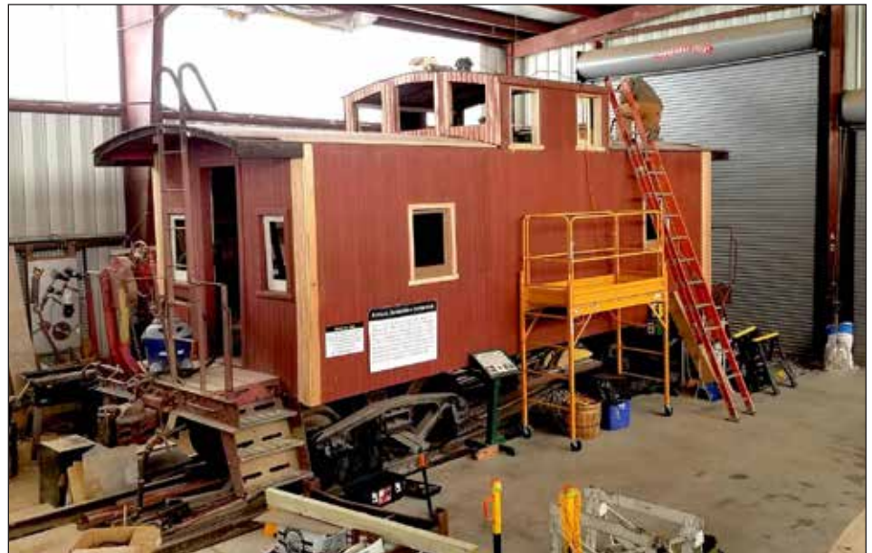
TOP LEFT: Volunteer Charlie Marks makes repairs to roof of the BR&P caboose on March 4, replacing rotten boards as suggested by our roofing contractor. Once exterior repairs to the body are complete, and new windows are installed, the museum will be seeking funds to have a durable membrane roof installed. TOP RIGHT: Jeremy Tuke installs a “new old stock” lockset on the bathroom door inside the caboose. ABOVE LEFT: Volunteer Justin Miciilo is replacing some of the modern hardware with more period correct peices on February 25. ABOVE RIGHT: Progress continues at a steady pace to complete body repairs and make the caboose weathertight so that it can leave its long-time home in the shop and make room for another project.
