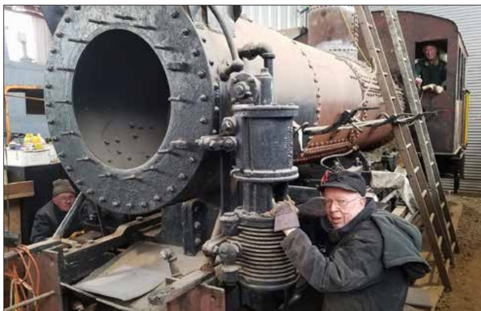
The cleanup of Brooklyn Navy Yard No. 12 has begun, thanks to Rand Warner (left), Norm Shaddick (right), and project leader Joel R. Shaw (inside the cab). One of the goals of this long-term cosmetic restoration project is to clean all components and inspect for damage prior to reassembly. The Steam Team can usually be found working each Saturday morning, and they invite you to join them.
