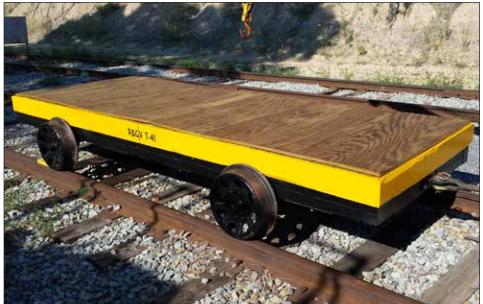
ABOVE and LEFT: Trailer T-41 was placed on live rail in July and currently serves as a boom tender for our Fairmont crane. The 12-foot trailer is ideal for carrying ties, tools, and other materials to aid in track maintenance around our museum property. The trailer was consisted of a volunteer team consisting of Norm Shaddick and Rand Warner, led by project manager Joel Shaw.
