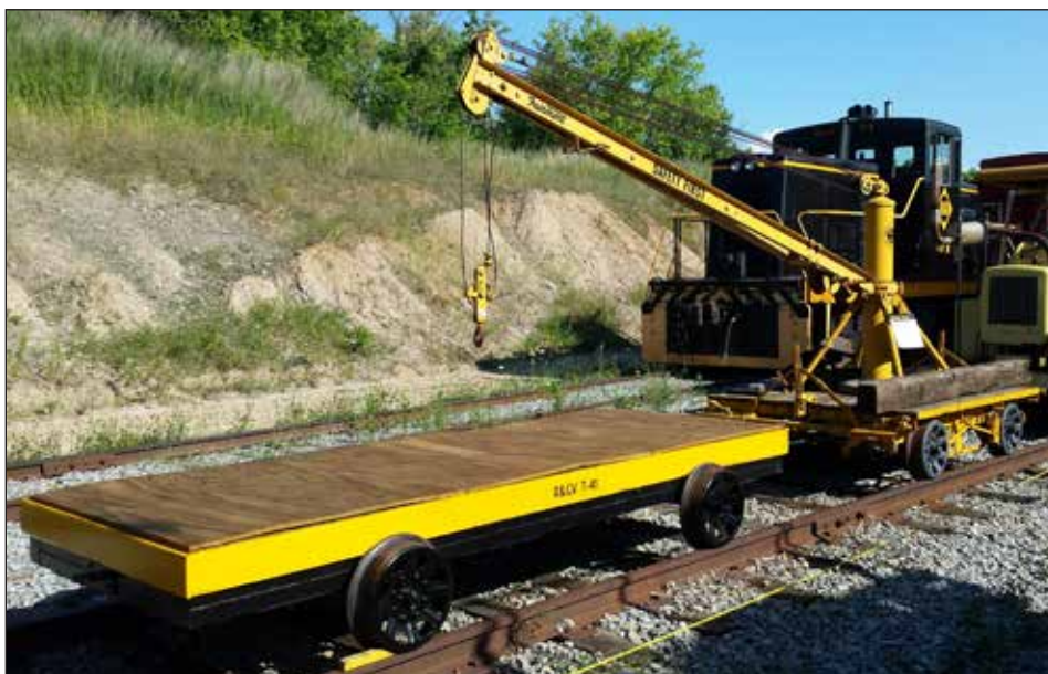
ABOVE and LEFT: Trailer T-41 was placed on live rail in July and currently serves as a boom tender for our Fairmont crane. The 12-foot trailer is ideal for carrying ties, tools, and other materials to aid in track maintenance around our museum property. The trailer was consisted of a volunteer team consisting of Norm Shaddick and Rand Warner, led by project manager Joel Shaw.
