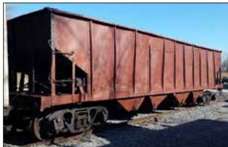
THE GREAT PAINT PROJECT: Two of our steel freight cars got a fresh coat of paint to help stabilize the structure and improve their appearance. MDT refrigerator car No. 12549 was built in 1953 and acquired in 1997, while PRR hopper car No. 747803 was built in 1909 and acquired in 1998. The majority of work was performed over four weekends. The cars will be returned to Track 6 by the end of the month. While this was not a restoration project, lettering may be applied to these cars in the future to further enhance their appearance. Thanks to all the volunteers who helped check this off the list!
