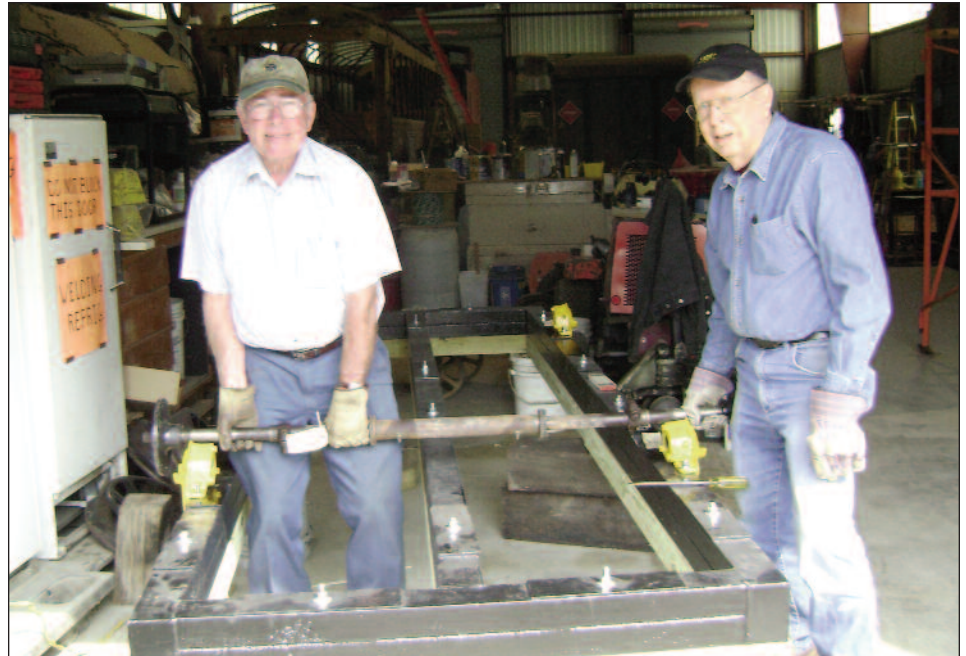
Construction of our third track car trailer continues, with the mounting of the axle to the frame, seen here with volunteers Rand Warner and Norm Shaddick. This new trailer will help enhance track car operations for next season. JOEL R. SHAW PHOTO
