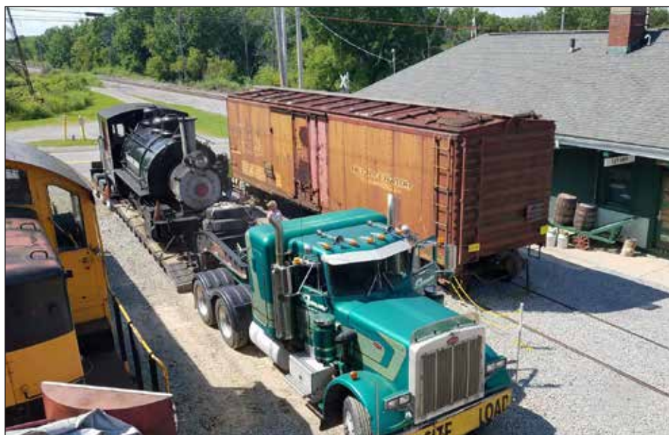
Viscose Co. No. 6 arrived on Monday, August 14. The engine is transported on a special trailer which allows the engine to be rolled on and off the tracks.
