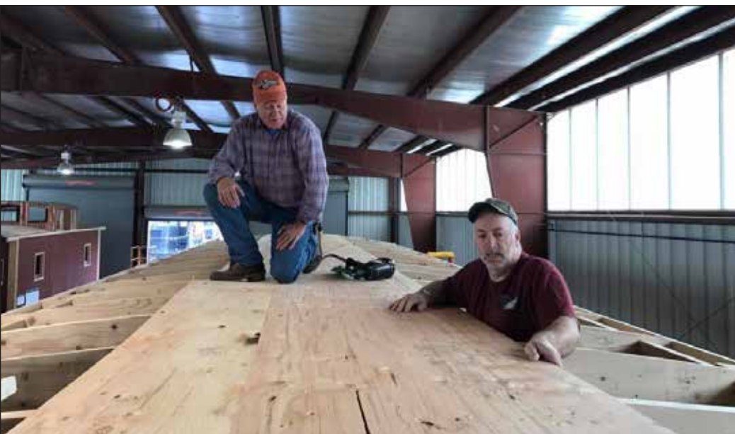
ABOVE: New volunteers Wayne McIntyre and Ron Conrad applied plywood sheathing to the roof of the open-air flatcar on May 6. RIGHT: and BELOW David Kehrer volunteered to complete the primer coat on the west side of the Pennsylvania Railroad railway post office car during the second week of April. The car will be cleaned and primed this spring in a project headed up by Kehrer. This project is looking for volunteers if you're willing to help! The RPO car also houses a signal technology display slated to open in June.
