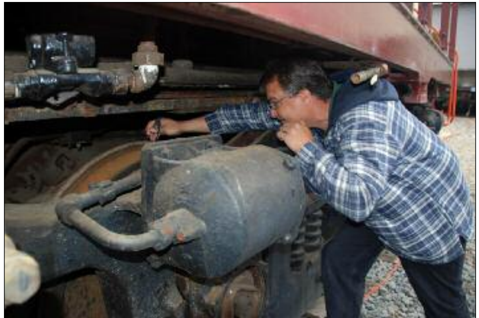
CLOSE QUARTERS: Chapter volunteer Jeff Carpenter performs inspections on Lehigh Valley 211. At left, Jeff is under the locomotive inspecting one of the traction motors. At right, he is using a wheel gauge to test tolerances and check the flange thickness. PHOTO BY DAVID SCHEIDERICH
