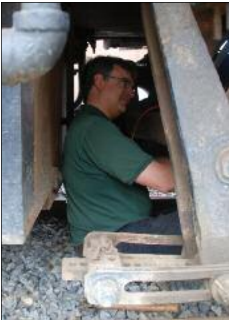
CLOSE QUARTERS: Chapter volunteer Jeff Carpenter performs inspections on Lehigh Valley 211. At left, Jeff is under the locomotive inspecting one of the traction motors. At right, he is using a wheel gauge to test tolerances and check the flange thickness. PHOTO BY DAVID SCHEIDERICH
