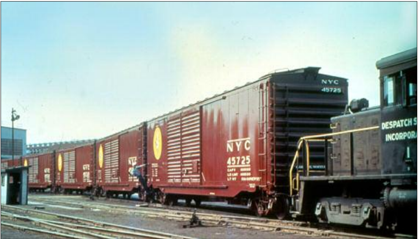
DESPATCH SHOPS: DSI switcher No. 1 pulls a string of brand new 50-foot double-door boxcars in fresh “Early Bird” paint. Despatch Shops built freight cars of all kinds for the New York Central and other railroads until 1970. The shop was constructed by Merchants Despatch Transport in 1897 in a section of town that was largely considered to be part of Penfield. The facility was originally built to support the operation and maintenance of the company’s fleet of refrigerated boxcars, and later expanded to manufacture freight cars for the railroads and other companies. The arrival of the carshops brought in hundreds of workers and their families who then settled a new community named “Despatch.” The first rail car to be built at Despatch was a refrigerator car completed on March 29th, 1898. By 1899 about 700 workers were employed with six buildings completed. Meanwhile the town was taking shape. In 1906 the village of Despatch was incorporated. In March of 1908 the village trustees renamed the thriving community “East Rochester.” Work continued at Despatch Shops, which was acquired and made a subsidiary of the New York Central Railroad. The New York Central provided the shop with its own locomotives (lettered for the shop facility), a tradition that continued on to the Penn Central days. Citing rising costs and other factors, Penn Central closed the shop in 1970. The MDT name would survive as a separate company that continues to lease freight cars and trailers to this day. PORTIONS QUOTED FROM DON SHILLING, PHOTO COLLECTION OF JOHN STEWART
