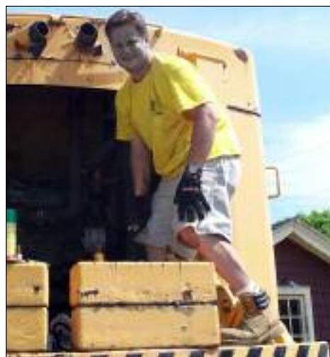
Chapter volunteer Chris Hauf works on the BE 22B Truck Crane on Saturday, June 7th. After draining many gallons of varnish-like gasoline and several hours of preparation work the upper motor hummed to life. The lower drive motor also was run after some tinkering with the fuel system. PHOTO BY JEREMY TUKE
