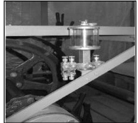
**Above** With a gas-mechanical chain drive locomotive, keeping your chains properly oiled is a must. To insure our Plymouth BL's chains stay lubricated, Kevin Klees has fabricated this chain oiler setup which will feed brushes mounted on the various drive chains. [Chris Hauf photo and caption]
