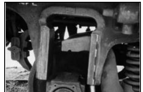
Close-up showing journal dropped out of truck. [Photos/captions by Bob Achilles]
