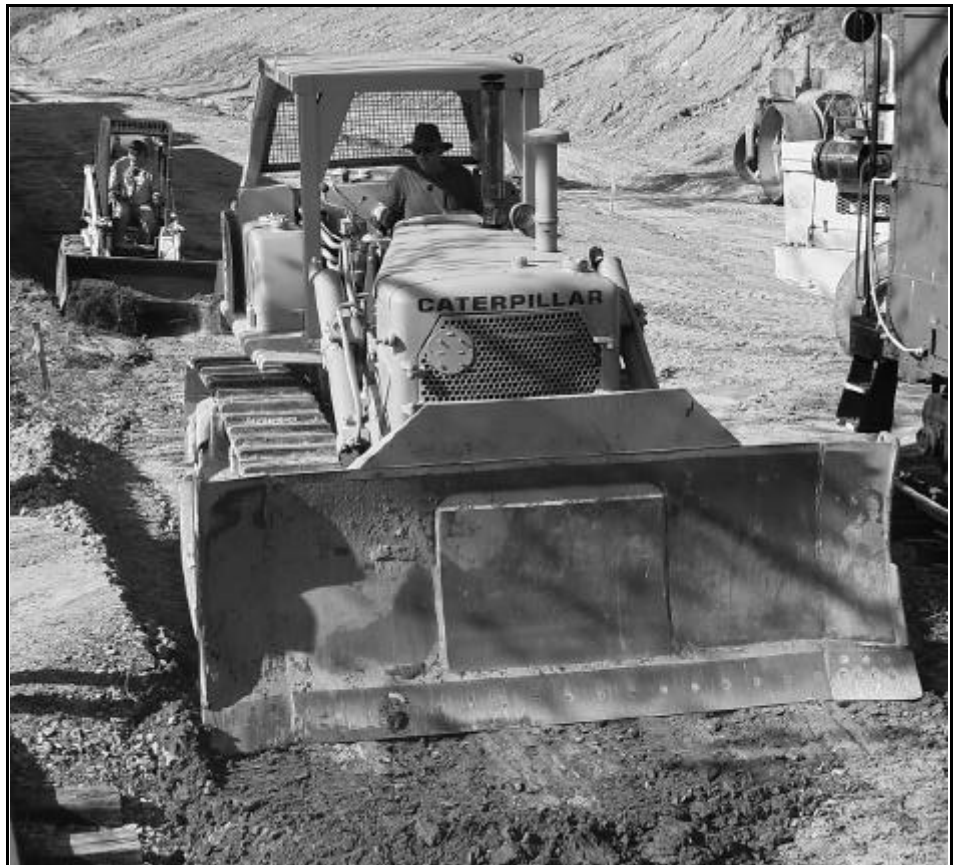
The museum's Cat D-7E dozer handles a little additional earth moving near the northeast corner of the Restoration Building with the museum's new (to us) Bobcat skid steer loader following along doing a little clean-up. [Chris Hauf photo]
