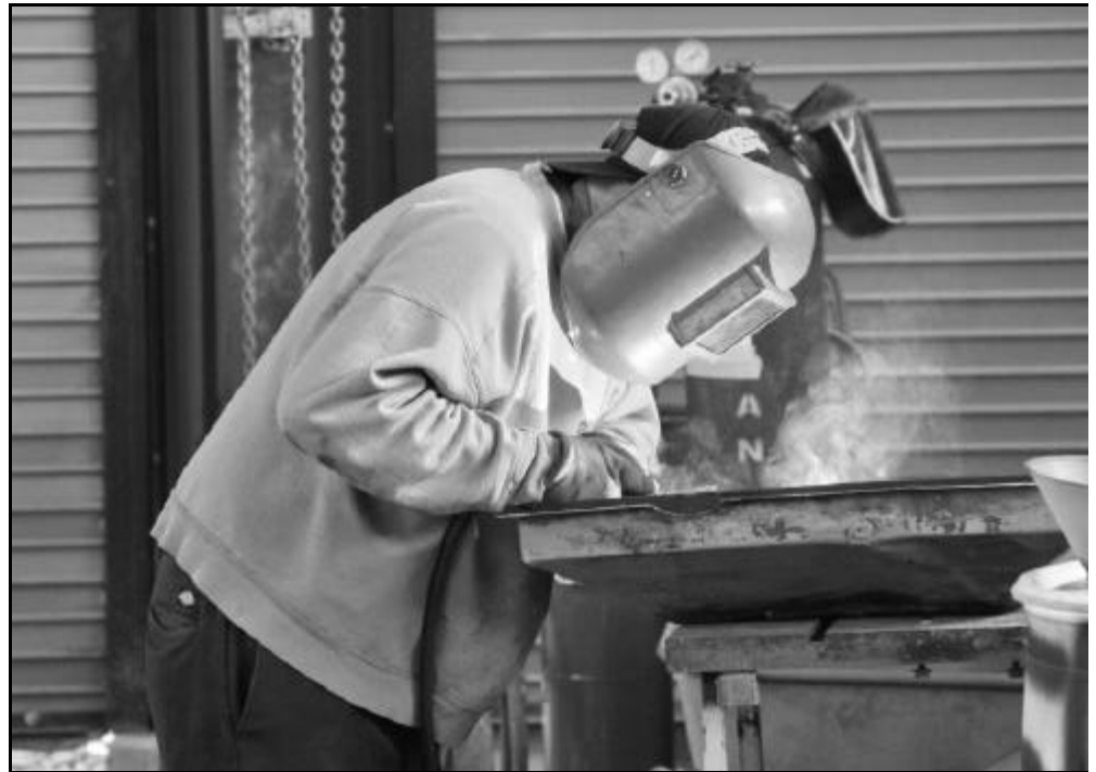
With connected track planned for this summer, the R&GVRR Museum hope to be able to move its restored Burro Model 40 crane out of the Restoration Building for use in the museum's demonstration railroad. One of the final steps to get this unit running is to complete some welding on the transmission oil pan. Art Mummery has that welding work well underway. [Chris Hauf photo & caption]
