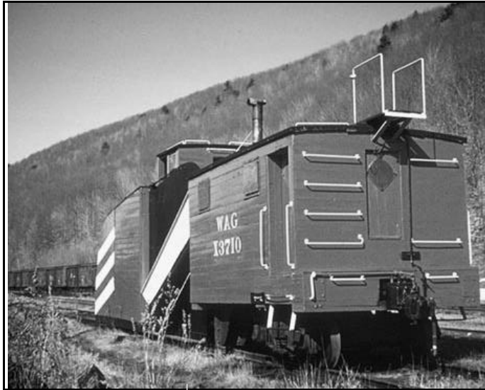
This view of the back portion of the WAG plow X3710 (B&M X3315), equipped with roof step and chimney. The paint scheme was a bright red, black, and white/cream trim. [Photo from John Stewart/NRHS archives]
