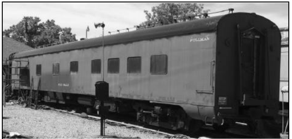
Pine Falls now has a shiny roof that should eliminate those roof leaks! [Chris Hauf photo]
