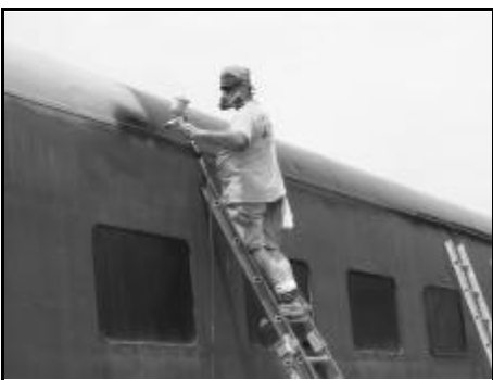
Chris Hauf is applying the final (black) paint using our HVLV spray equipment [Gale Smith photo]
