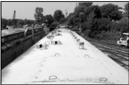
The roof after receiving a primer coat of paint. [Chris Hauf photo]
