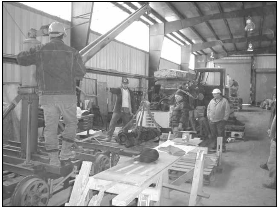
The Fairmont Track Crane being used to move the Buda engine block. (Ron Amberger photo)
