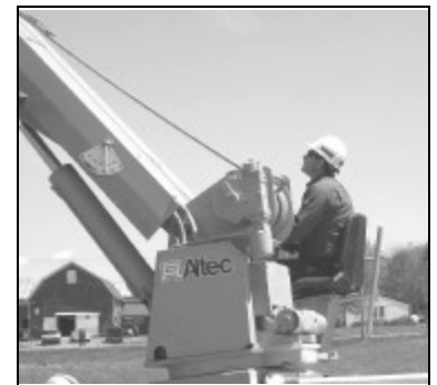
Left, above: Combination crawler crane, auger setting a pole.
